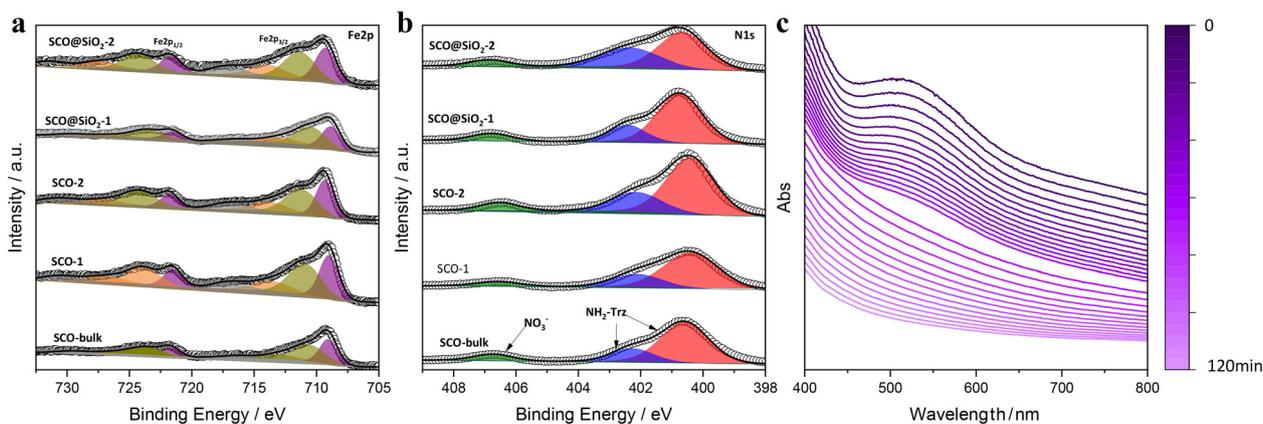
**Fig. 2** Spectra from XPS of Fe 2p (a) and N 1s (b) of the different NPs and the bulk. (c) Dependency of the UV-vis absorbance of SCO@SiO<sub>2</sub>-1 redispersed in water as a function of time.
