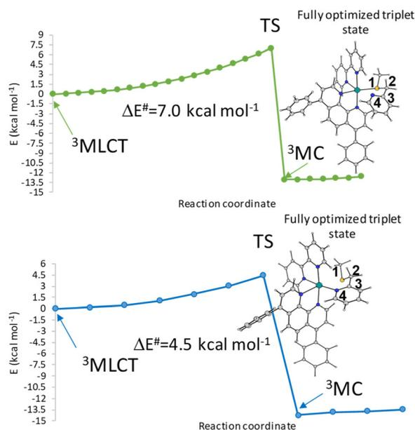
**Fig. 3** Relaxed potential energy scans from the  $^3\text{MLCT}$  state to  $^3\text{MC}$  (a) Tc and (b) Td of the Ru complex calculated by varying the S1–C2–C3–N4 and N4–C3–C2–S1 dihedral angles ( $^\circ$ ).
