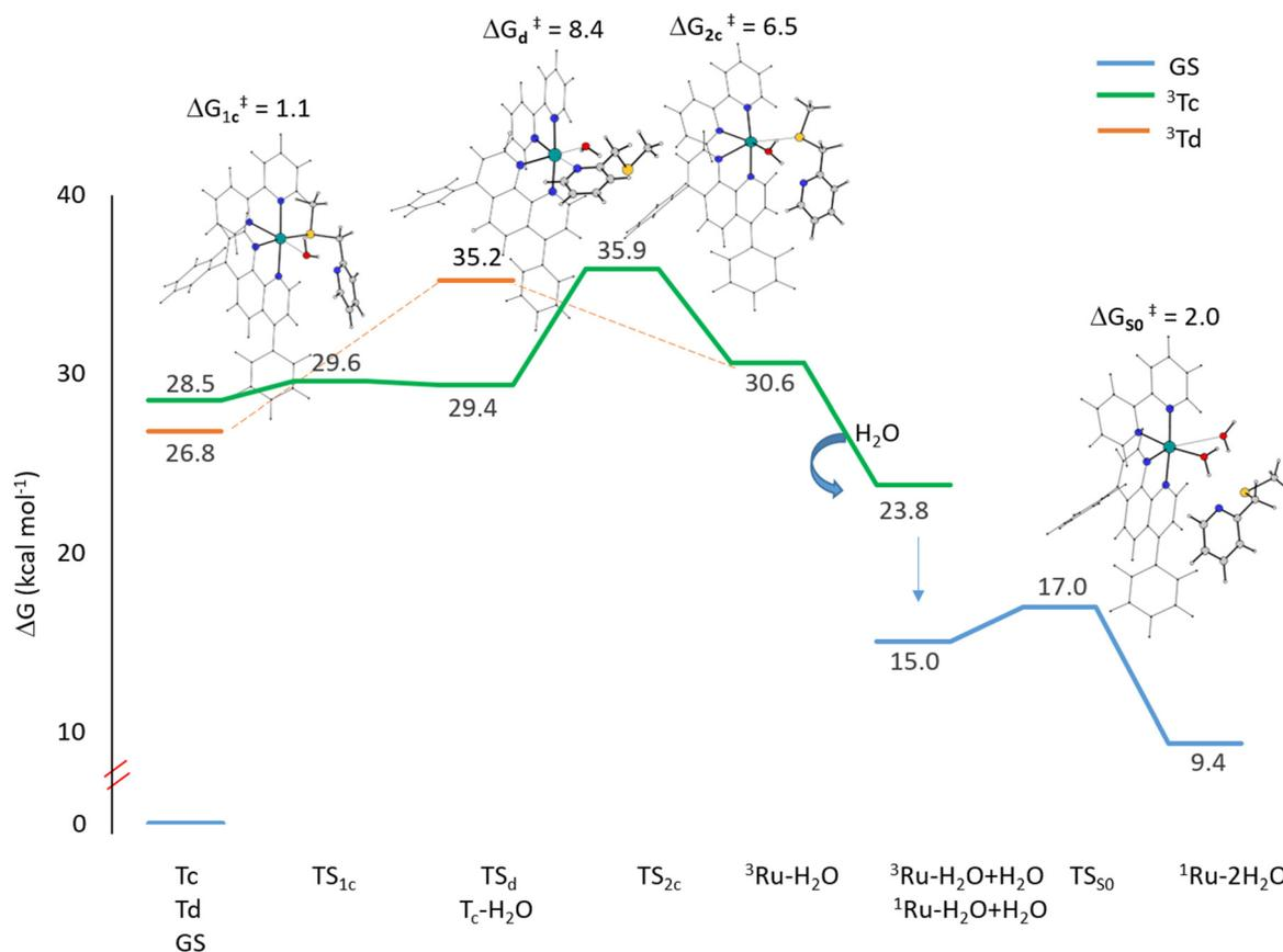
**Fig. 6** Calculated free energy profiles in water describing the light-induced substitution mechanism of the Ru complex. Relative energies are in  $\text{kcal mol}^{-1}$  and calculated with respect to the ground state singlet energy of the complex.
