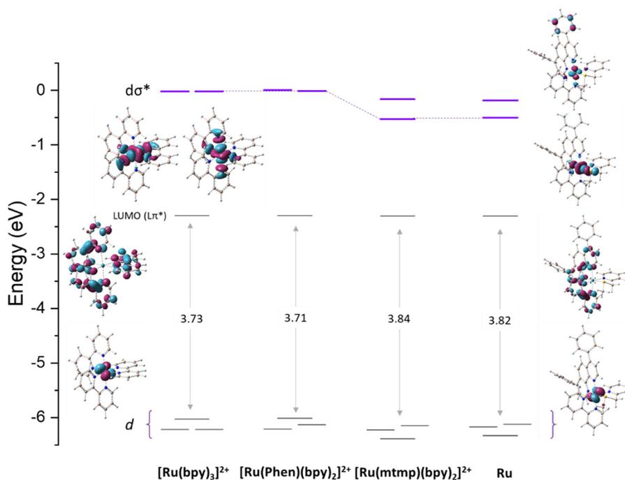
**Fig. 5** Energy diagram of the molecular orbitals of the Ru complex compared with those of [Ru(bpy)<sub>3</sub>]<sup>2+</sup>, [Ru(phen)(bpy)<sub>2</sub>]<sup>2+</sup> (phen = phenanthroline), and [Ru(mtmp)(bpy)<sub>2</sub>]<sup>2+</sup> with representative plots of HOMOs, LUMOs and dσ\* orbitals.
