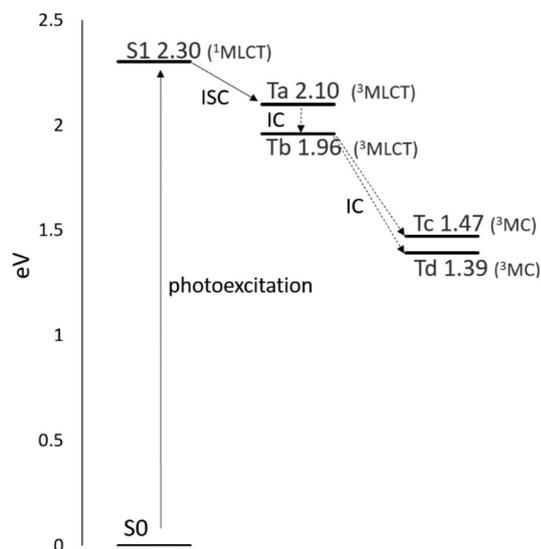
**Fig. 4** Simplified Jablonski diagram depicting the key photophysical processes for the Ru complex: photoexcitation, intersystem crossing (ISC), and internal conversion (IC). The diagram highlights that  $^3\text{MC}$  states fall below the  $^3\text{MLCT}$  states.
