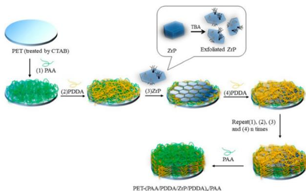
**Fig. 13** Schematic of the layer-by-layer (LbL) assembly for polyacrylic acid (PAA)/poly(dimethyl diallyl ammonium chloride) (PDPA)/zirconium phosphate (ZrP)/PDPA quadlayers. PET: polyethylene terephthalate; TBA: tetrabutylammonium; CTAB: hexadecyl trimethyl ammonium bromide. Reproduced with permission from ref. 218, Copyright 2018 MDPI.
