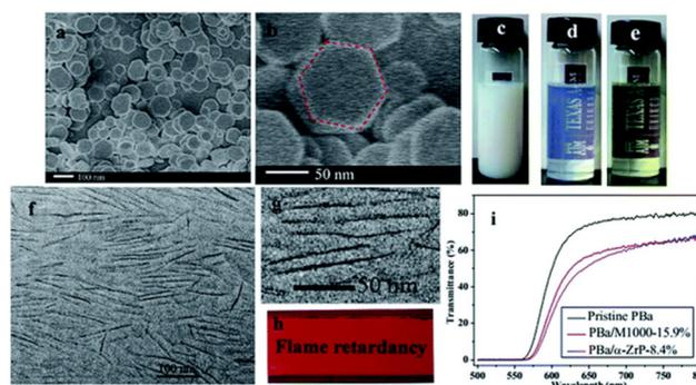
Fig. 11 (a) and (b) SEM of original  $\alpha$ -ZrP, (c) original  $\alpha$ -ZrP in acetone, (d) exfoliated  $\alpha$ -ZrP in acetone, (e) Ba/ $\alpha$ -ZrP-8.4% in acetone, (f) and (g) TEM of PBa/ $\alpha$ -ZrP-8.4% nanocomposites, (h) photographic images of PBa/ $\alpha$ -ZrP-8.4% nanocomposites and (i) light transmission spectra of samples. Adapted with permission from ref. 209, Copyright 2016 Royal Society of Chemistry.
