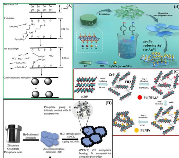
**Fig. 6** Schematic illustration of preparation steps of the catalysts: (A) Ni/ZrP adapted with permission from ref. 24, Copyright 2018 American Chemical Society; (B) ZrP@PDA/AuNP or ZrP@PDA/AuNP, adapted with permission from ref. 30, Copyright 2020 MDPI; (C) ZrP-PdNPs, adapted with permission from ref. 31, Copyright 2022 Taiwan Institute of Chemical Engineers; (D) Pt/ZrP. Adapted with permission from ref. 36, Copyright 2023 John Wiley and sons.
