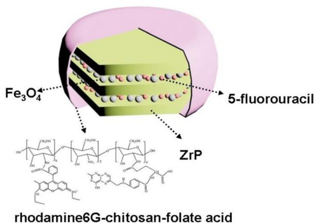
**Fig. 9** Schematic representation of the 5-FU/Fe<sub>3</sub>O<sub>4</sub>/α-ZrP@CHI-FA-R6G nanocomposites. Reproduced with permission from ref. 177, Copyright 2015 American Chemical Society.
