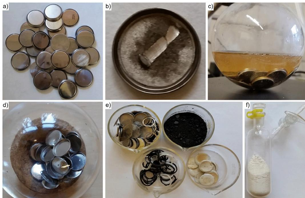
**Fig. 1** Post-consumer Li–MnO<sub>2</sub> batteries used for synthesizing lithium aryloxides (a); coin cell cap with the lithium anode (b); reaction mixture (c); anode caps after the reaction (d); stainless steel, plastic, and cathode material recovered from the reaction (e); and isolated crystalline lithium aryloxide [Li<sub>6</sub>(OAr)<sub>6</sub>] (f).
