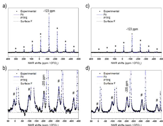
**Fig. 1**  $^{19}\text{F}$  NMR spectra of fluorinated NCA samples (all samples contain 6 wt% of PTFE as an internal reference, and its main peak is indicated by the grey arrow): NCA-F1 (a), and a zoom-in view of the LiF-type signature (b), NCA-F2 (c), and a zoom-in view of the LiF-type signature (d). \*/# mark spinning sidebands for PTFE and LiF signals, respectively.
