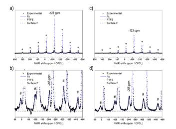
Fig. 1 <sup>19</sup>F NMR spectra of fluorinated NCA samples (all samples contain 6 wt% of PTFE as an internal reference, and its main peak is indicated by the grey arrow): NCA-F1 (a), and a zoom-in view of the LiF-type signature (b), NCA-F2 (c), and a zoom-in view of the LiF-type signature (d). \*/# mark spinning sidebands for PTFE and LiF signals, respectively.
