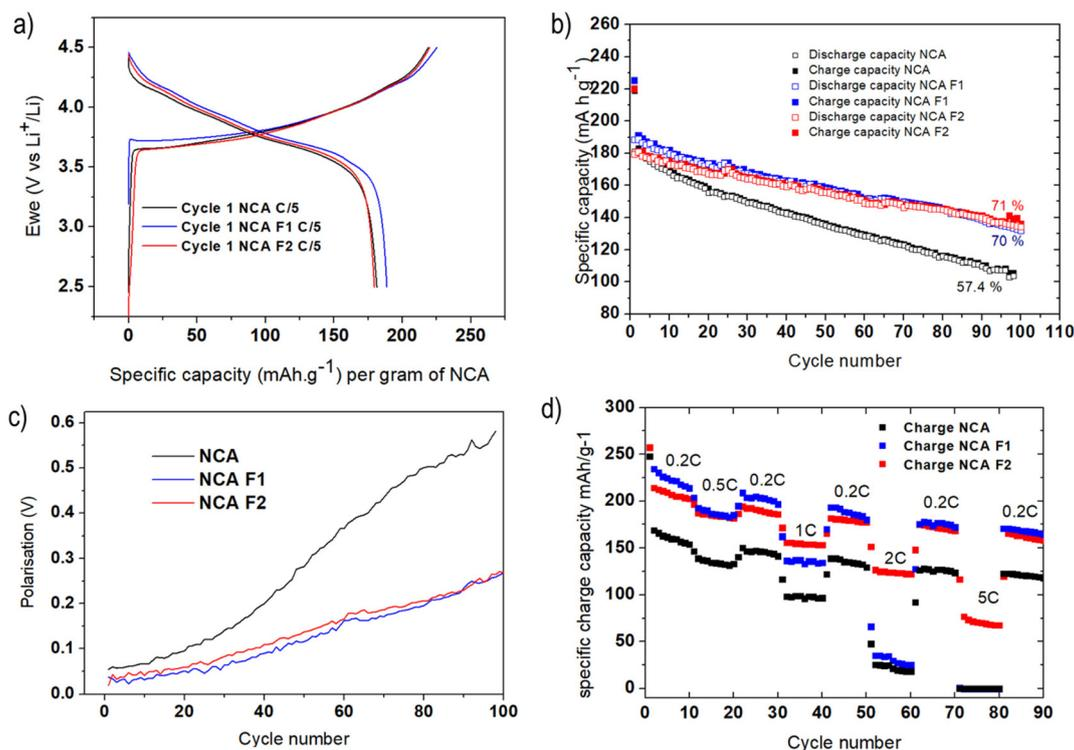
**Fig. 3** Galvanostatic voltage profiles of NCA/Li, NCA-F1/Li, and NCA-F2/Li cells cycled at C/5 between 4.5 and 2.5 V versus Li<sup>+</sup>/Li; the first cycle is displayed (a); specific charge capacity of NCA/Li, NCA-F1/Li, and NCA-F2/Li cells cycled at C/5 (b); polarisation as a function of the cycle number for NCA, NCA-F1 and NCA-F2 cells (c); and current rate capability of NCA, NCA-F1, and NCA-F2 electrodes (d).
