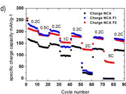
Fig. 3 Galvanostatic voltage profiles of NCA/Li, NCA-F1/Li, and NCA-F2/Li cells cycled at C/5 between 4.5 and 2.5 V versus Li<sup>+</sup>/Li; the first cycle is displayed (a); specific charge capacity of NCA/Li, NCA-F1/Li, and NCA-F2/Li cells cycled at C/5 (b); polarisation as a function of the cycle number for NCA, NCA-F1 and NCA-F2 cells (c); and current rate capability of NCA, NCA-F1, and NCA-F2 electrodes (d).
