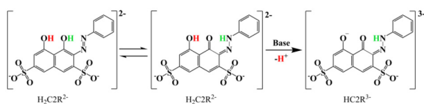
Scheme 1 Resonance forms of H 2 C 2 R 2- and its monodeprotonated form HC 2 R 3- .
