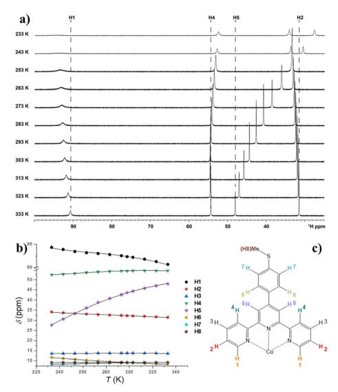
Fig. 6 Panel a: <sup>1</sup>H-NMR spectra of an acetonitrile-d<sub>3</sub> solution of **1** acquired at different temperatures (dashed lines indicates the chemical shifts assignment). Only selected resonances are shown for clarity. Panel b: Temperature dependence of the chemical shifts of every non-equivalent hydrogen of **1**. Lines are the best fitting curves, whose function and parameters are described in the text. Panel c: <sup>1</sup>H assignments for the *TerpyPhSMe* ligand in **1**.
