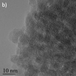
Fig. 6 BF-TEM with SAED (a) and HR-TEM of TiO2@C (b).
