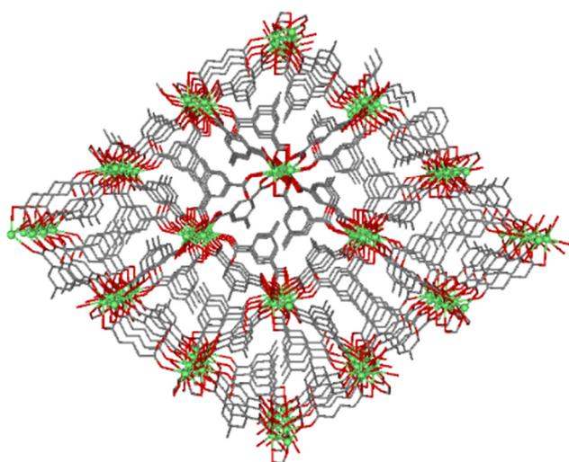
**Fig. 1** Perspective view of **GR-MOF-17** along the *a* axis. Ce atoms are represented in green, carbon atoms are represented in grey, oxygen atoms are represented in red and hydrogen atoms were omitted for clarity.
