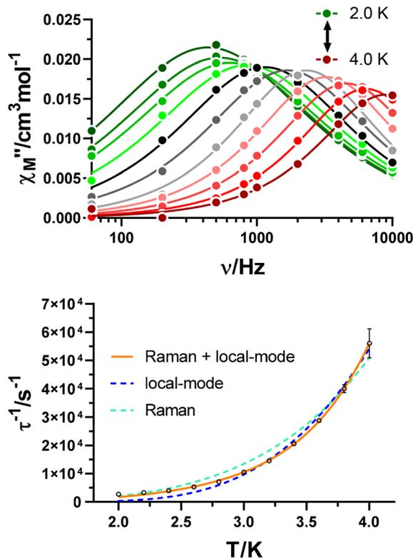
**Fig. 6** Variable-temperature frequency dependence of the  $\chi''_M$  signal under a 1 kOe applied field for GR-MOF-18 (top). Dependence of the inverse of the relaxation time on the temperature (bottom).
