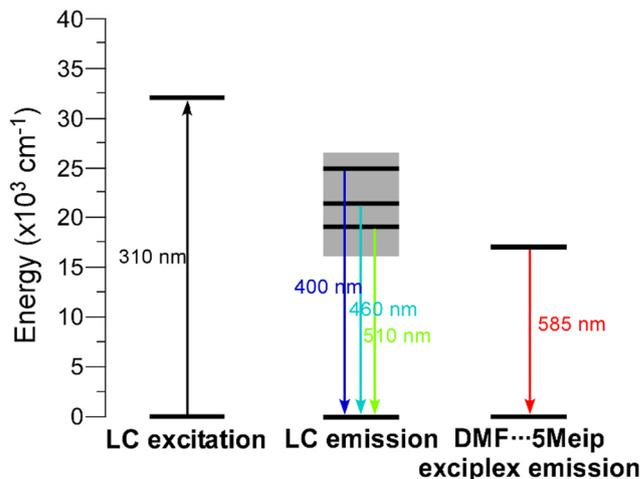
**Scheme 1** Energy diagram showing the most relevant excitation and emission band maxima observed for compounds **GR-MOF-17** and **GR-MOF-18**. Note that the wavelengths are rounded in an effort to represent the band maxima of both compounds.
