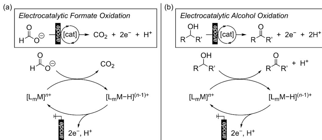
**Scheme 1** General scheme for electro-oxidation of (a) formate, or (b) alcohols *via* a metal–hydride intermediate.
