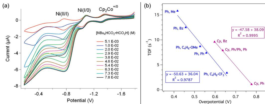
**Fig. 2** (a) CVs of **1e** in benzonitrile showing electrocatalytic formate oxidation. Adapted with permission from ref. 45. Copyright 2011 American Chemical Society. (b) Correlation between TOF and overpotential for electrocatalytic formate oxidation with **1a–1h**. Data labels indicate the P<sub>2</sub>N<sub>2</sub>R<sup>R'</sup> R and R' substituents, respectively. Adapted with permission from ref. 52. Copyright 2018 American Chemical Society.
