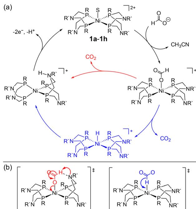
**Scheme 3** (a) Proposed mechanisms for formate oxidation by **1a-1h**. (b) Proposed transition states via  $\beta$ -deprotonation (red, left) or direct hydride transfer (blue, right).<sup>45,46,54</sup>
