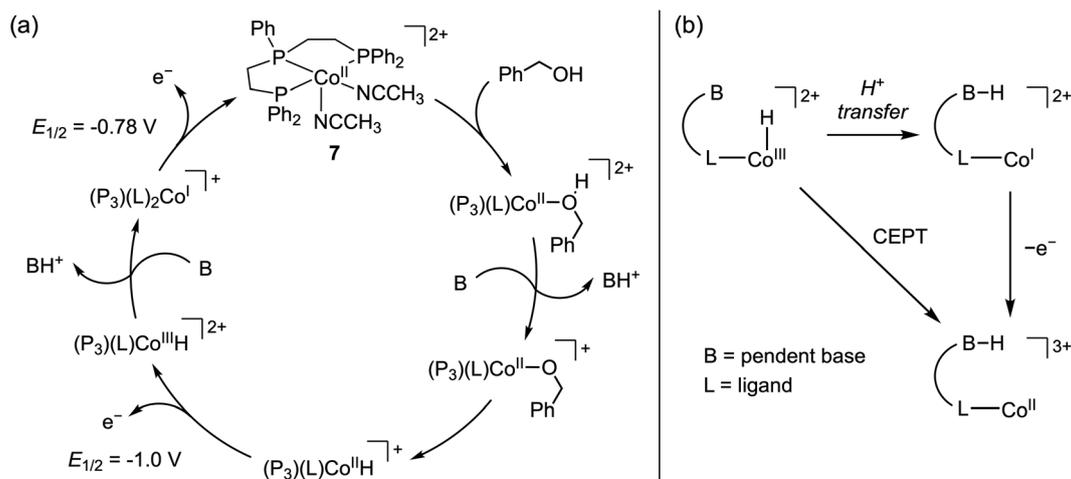
**Scheme 5** (a) Proposed mechanism for benzyl alcohol oxidation by **7** with  $i\text{Pr}_2\text{EtN}$ .<sup>80</sup> (b) Possible ligand-promoted concerted electron-proton transfer (CEPT) pathway for Co(III)-hydride oxidation.
