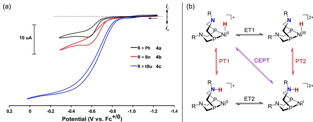
**Fig. 4** (a) CVs of **4a–4c** in acetonitrile showing electrocatalytic oxidation of benzyl alcohol in the presence of triethylamine. Adapted from ref. 59 with permission from the Royal Society of Chemistry. (b) Possible PCET pathways for Ni( $\text{P}_2\text{N}_2$ )-hydride oxidation. Adapted with permission from ref. 61. Copyright 2022 American Chemical Society.
