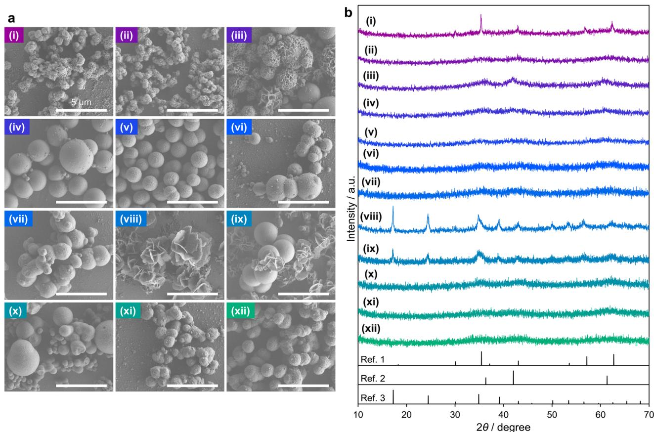
**Fig. 1** SEM images (a) and XRD patterns (b) of products (i)–(xii) corresponding to entries 1–12 in Table 1, respectively. Scale bars of SEM images (a) are 5  $\mu\text{m}$ . Black lines in (b), ref. 1, 2, and 3, correspond to reference diffraction peak positions of cubic  $\text{Fe}_3\text{O}_4$  (PDF#00-001-1111), cubic  $\text{FeO}$  (PDF#00-001-1223), and cubic  $\text{Co}(\text{Fe}(\text{CN})_5\text{NO})\cdot 5\text{H}_2\text{O}$  (PDF#00-043-0768), respectively.
