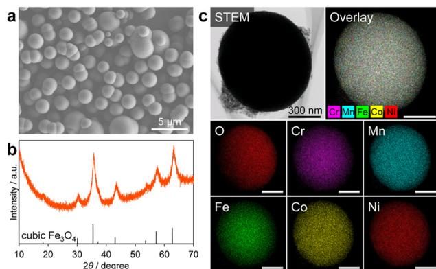
**Fig. 2** SEM image of a precursor composite (before calcination, a). An XRD pattern (b), and STEM and EDX mappings (c) of HE-MARIMO (after calcination). The black lines in (b) correspond to reference diffraction peak positions of cubic  $\text{Fe}_3\text{O}_4$  (PDF#00-001-1111). An overlay image in (c) created by merging EDX mapping images of Cr, Mn, Fe, Co, and Ni. Scale bars of STEM and EDX mapping images (c) are 300 nm.
