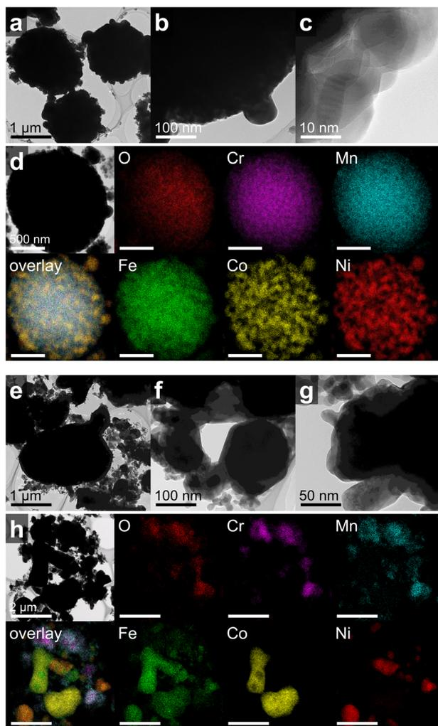
**Fig. 5** TEM images (a–c), STEM and EDX mapping images (d) of the spent HE-MARIMO. Scale bars of EDX mapping images (d) are 500 nm. TEM images (e–g), and STEM and EDX mapping images (h) of spent sss-composite. Scale bars of EDX mapping images (h) are 2  $\mu$ m.
