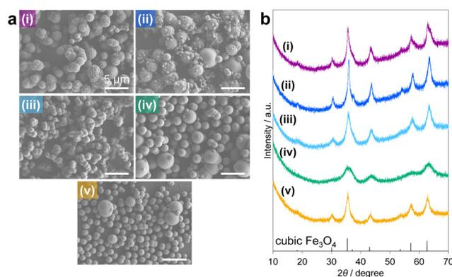
**Fig. 6** SEM images (a) of precursor composites (before calcination) and XRD patterns (b) of quaternary MARIMOs (after calcination). (i–v) correspond to Cr-free, Mn-free, Fe-free, Co-free, and Ni-free MARIMOs, respectively. Scale bars of SEM images (a) are 5  $\mu\text{m}$ . The black lines in (b) correspond to reference diffraction peak positions of cubic  $\text{Fe}_3\text{O}_4$  (PDF#00-001-1111).
