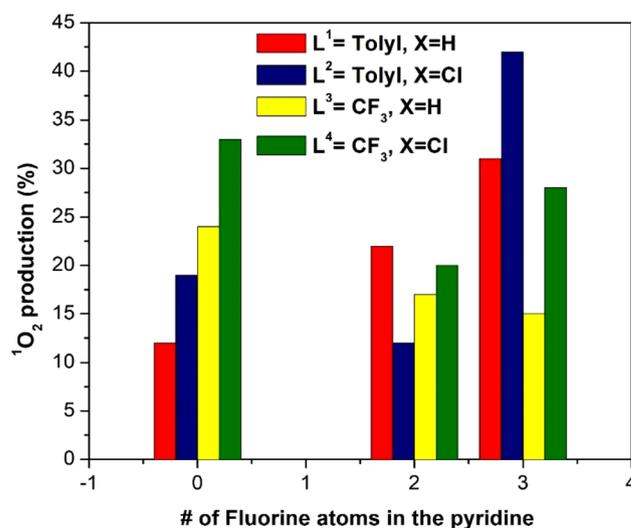
**Fig. 4** Plot of singlet oxygen production quantum yield,  $\Phi_{\Delta}$ , of the (N<sup>^</sup>N<sup>^</sup>N<sup>^</sup>)Pt(pyF) complexes as a function of the N<sup>^</sup>N<sup>^</sup>N<sup>^</sup> ligand and the pyridine used.
