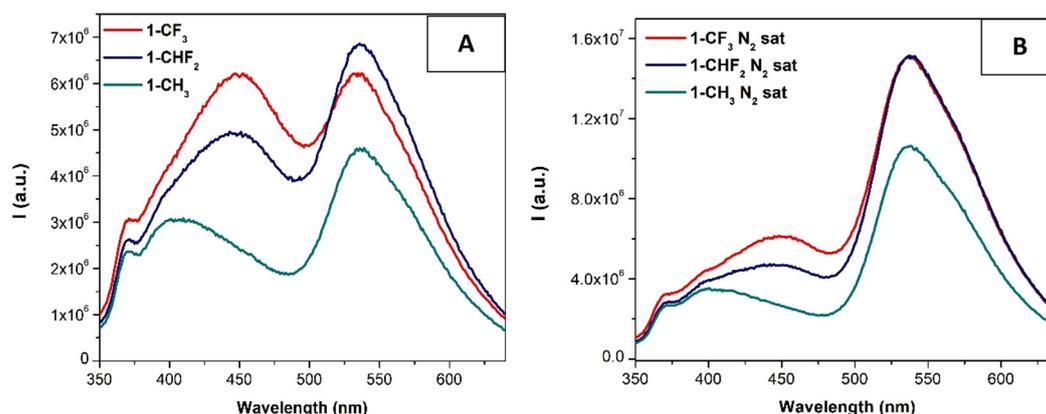
**Fig. 2** Emission spectra of compounds **1-CF<sub>3</sub>**, **1-CHF<sub>2</sub>** and **1-CH<sub>3</sub>** in  $10^{-5}$  M air-eq. (A) and  $\text{N}_2$  sat. (B) DMSO solutions ( $\lambda_{\text{exc}} = 330$  nm), respectively.
