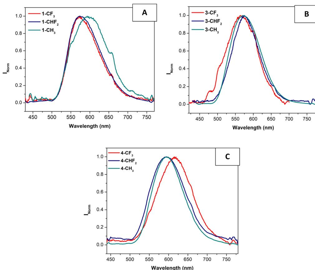
**Fig. 3** Normalized emission spectra of compounds  $x$ -CF<sub>3</sub>,  $x$ -CHF<sub>2</sub> and  $x$ -CH<sub>3</sub> ( $x = 1$ , A;  $x = 3$ , B and  $x = 4$ , C) in the solid-state ( $\lambda_{exc} = 400$  nm).
