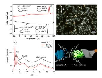
Fig. 16 DSC curve, POM image, and PXRD spectra of LC [Cu<sub>4</sub>I<sub>4</sub>] cluster Schematic illustration of grinding-induced MCL activity. Reproduced from ref. 109 with permission. Copyright (2016), American Chemical Society
