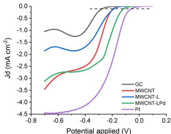
Fig. 8 ORR electrocatalytic performance, LSV 1600 rpm rotation rate, and  $5 \text{ mV s}^{-1}$  scan rate in KOH 0.1 M  $\text{O}_2$  saturated solution. RRDE disk current densities of the modified GC electrode and the benchmark electrode. The horizontal dotted line at a current density of  $-0.1 \text{ mA cm}^{-2}$  shows the onset potential of samples.
