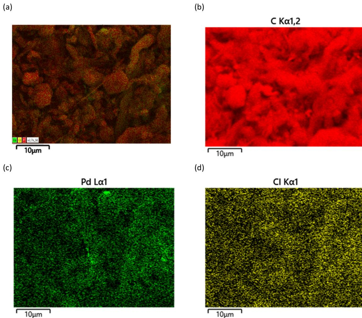
Fig. 7 EDS mapping of MWCNT-LPd: (a) EDS layered image, (b) C signals, (c) Pd signals, and (d) Cl signals.
