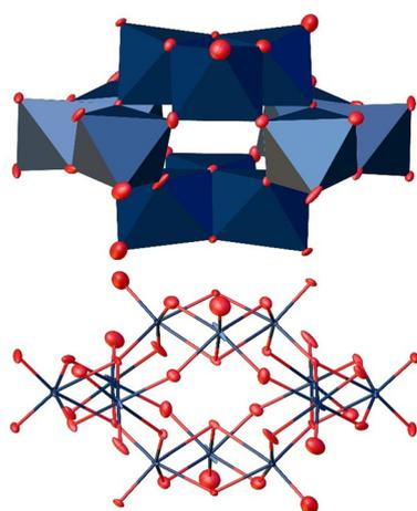
**Fig. 4** Solid-state structure of the anion  $[\text{W}_{12}\text{O}_{40}]^{8-}$  determined by scXRD. Polyhedra representation above and atom model bottom. The compound was crystallized in the triclinic space group  $P\bar{1}$  (2).  $R_1$ : 4.74%,  $wR_2$ : 9.47%,  $R_{\text{int}}$ : 4.76%,  $\text{Goof}$ : 1.078. Color code: blue: metal atoms (W), red: oxygen atoms. The .cif file is available in the CCDC database. Deposition number: 2293850.†
