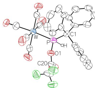
**Fig. 4** Molecular structure of **10a**. Thermal ellipsoids are set at 50% probability and hydrogen atoms are omitted for clarity except for the one bound to phosphorus. Selected bond lengths/Å and bond angles/°: W–P 2.452(3), P–O1 1.695(9), P–C1 1.915(12), O1–P–W 106.6(3), O1–P–C1 97.5(5), C1–P–W 130.6(4), C20–O1–P 124.0(9).
