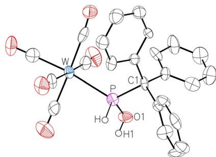
**Fig. 2** Molecular structure of **2**. Thermal ellipsoids are set at 50% probability and hydrogen atoms are omitted for clarity except for those bound to phosphorus or oxygen atoms. Selected bond lengths/Å and bond angles/°: W–P 2.527(3), P–O1 1.575(8), P–C1 1.919(10), O1–P–W 113.8(3), O1–P–C1 105.8(4), C1–P–W 124.1(3).
