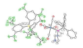
Fig. 6 Molecular structure of 11b. Thermal ellipsoids are set at 50% probability and solvent molecules and hydrogen atoms are omitted for clarity except for the one bound to phosphorus. Selected bond lengths/ Å and bond angles/°: W-P 2.4611(4), P-N1 1.7773(14), P-C5 1.9239(16), N1-P-W 113.30(5), N1-P-C5 102.46(7), C5-P-W 130.29(5).
