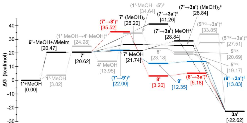
**Fig. 3** Computed [CPCM(tol)/PWPB95-D3/def2-QZVPP(ecp)//CPCM(tol)/PBEh-3c] Gibbs energy profile for the addition of methanol to model complex adduct **1**. Colour code used for  $S_N2$ - (grey) and  $S_N1$ -type mechanism with direct or MeOH-assisted H-transfer (black), *N*-Melm-assisted H-transfer (blue) or involving decomplexation/recomplexation (red).
