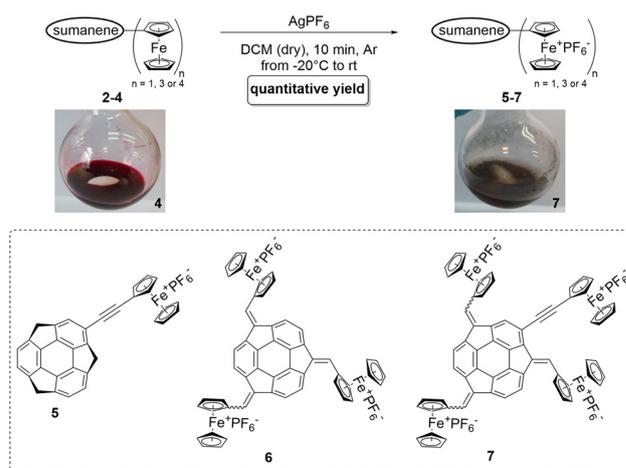
**Fig. 4** Oxidation of the sumanene-ferrocene conjugates **2–4** to  $\text{Fc}^+$ -containing compounds **5–7**. Solution colours before and after the reaction in the representative synthesis of **7** from **4** are also presented.
