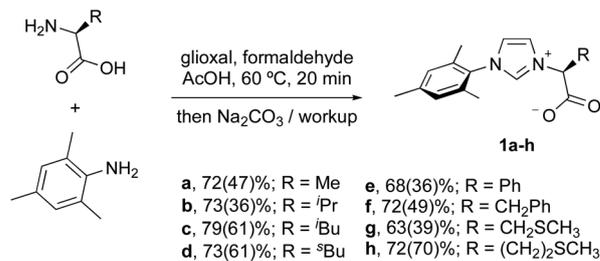
**Scheme 1** Synthesis of chiral zwitterionic imidazolium salts **1a–h**, and their corresponding selectivity (isolated yield) %.
