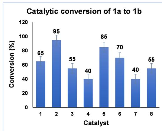
Fig. 4 Reduction of **1a** to **1b** by CH<sub>3</sub>NHNH<sub>2</sub> catalyzed by **1–8** (conversion percentage are the average values of three independent experiments within 3–5% error). Conversion percentages (%) were measured by <sup>1</sup>H NMR spectroscopy after addition of a specific amount of 1,3-dimethoxybenzene as internal standard.
