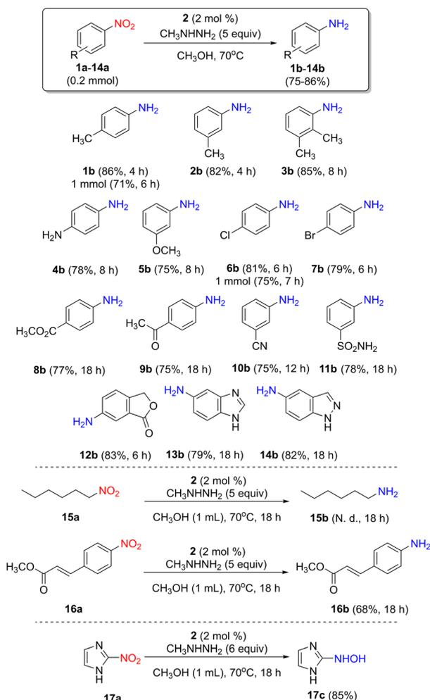
**Scheme 3** Chemoselectivity of the reduction of nitro-compounds **1a-16a** by  $\text{CH}_3\text{NHNH}_2$  to the corresponding amines **1b-14b** and **16b** as well as antibiotic **17a** to the corresponding *N*-hydroxylamine derivative **17c**, catalyzed by **2** (product isolated yield after column chromatography/appropriate time reported in parentheses). N. d. = not detected.
