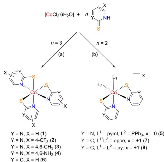
**Scheme 2** Synthetic schemes and structures of complexes  $[\text{Co}(\text{L}^{\text{NS}})_3]$  and  $[\text{Co}(\text{L}^{\text{NS}})_2\text{L}^1\text{L}^2]^{x+}$  (1–8): (a)  $(\text{CH}_3\text{CH}_2)_2\text{NH}$ , 50–70 °C for 3 h under atmospheric conditions, and (b) KOH or  $(\text{CH}_3\text{CH}_2)_2\text{NH}$  or  $\text{CH}_3\text{ONa}$ , 50–70 °C for 2 h under atmospheric conditions.
