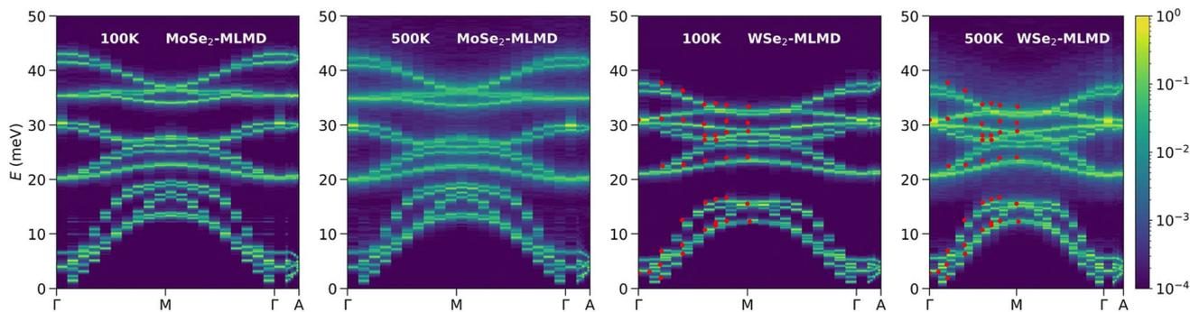
Fig. 13 Phonon spectral energy density calculated by Gupta *et al.*<sup>145</sup> for MoSe<sub>2</sub> and WSe<sub>2</sub> using molecular dynamics and MLIPs. The effects of anharmonicity can be clearly seen in the 500 K spectra as the broadening of the lines and the diffusive intensities. Reprinted with permission from Royal Society of Chemistry Copyright (2023).
