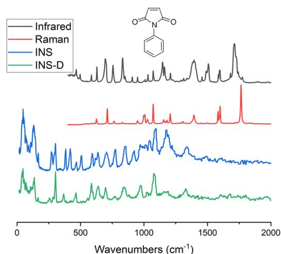
Fig. 2 Various experimental techniques used to measure vibrations. An example is shown for *N*-phenylmaleimide in this figure. INS-D in the legend refers to spectrum measured on partially deuterated *N*-phenylmaleimide (with the phenyl ring deuterated). Image produced using data published and provided by Parker.<sup>11</sup>
