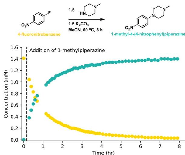
Fig. 4 Online HPLC monitoring of 1-methylpiperazine and 1-methyl-4-(4-nitrophenyl)piperazine.
