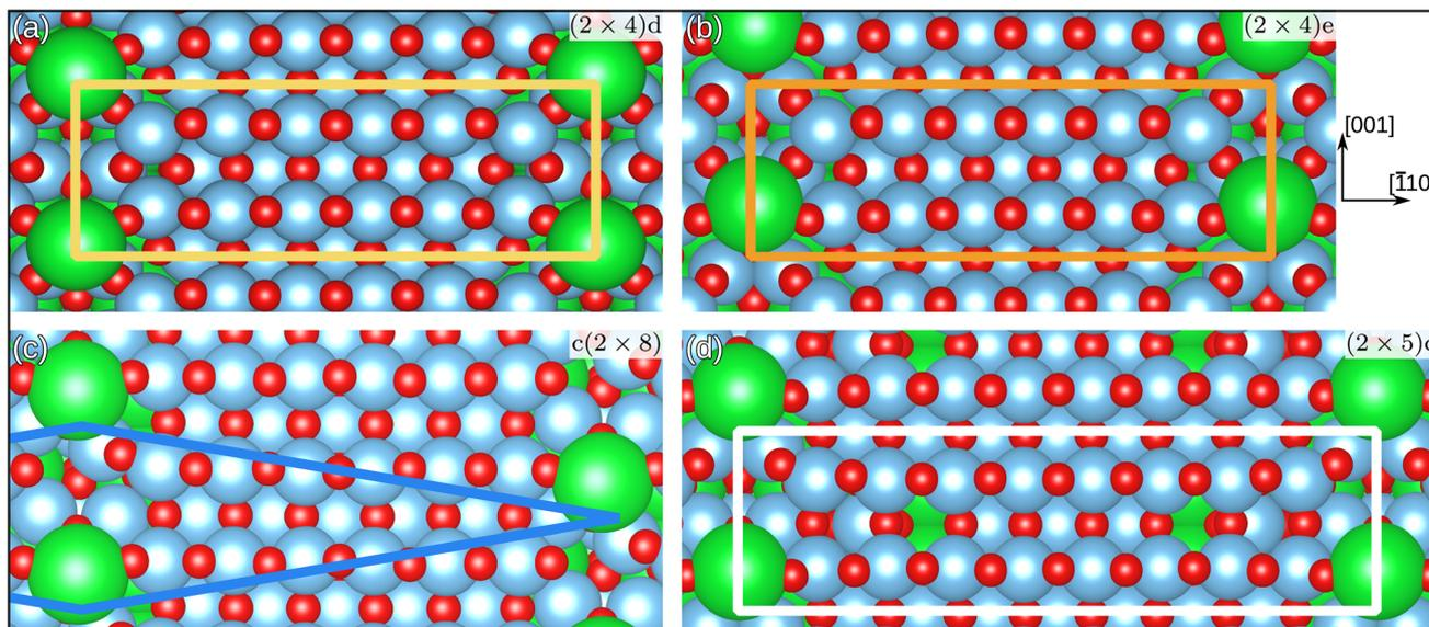
Fig. 4 Top view of SrTiO<sub>3</sub>(110) overlayer candidates. (a) and (b) with (2 × 4) bulk periodicity. (c) With centered (2 × 8) periodicity and (d) with (2 × 5) periodicity. The orange and white rectangles and the blue rhombus indicate (parts of) the respective unit cells. Only half of the c(2 × 8) unit cell is outlined. See Fig. S11 of the ESI† for the full picture.
