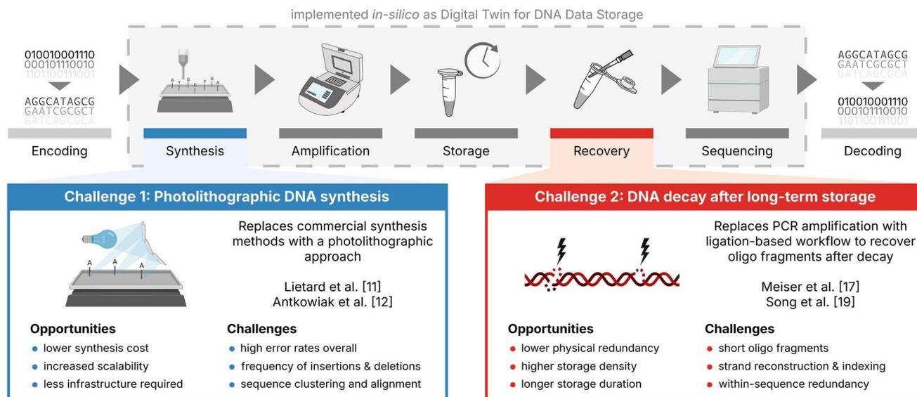
**Fig. 1** Current challenges in the DNA data storage workflow. Illustration of the current state-of-the-art DNA data storage workflow (top) with the two new additions discussed in this study highlighted: photolithographic synthesis (blue box) and DNA decay (red box). Both the state-of-the-art workflow and the challenges have been implemented *in silico* as a digital twin for DNA data storage (grey box, see also Gimpel *et al.*<sup>9</sup>) to support codec development and experimental planning.
