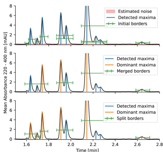
**Fig. 2** Visualized peak picking procedure on a representative chromatogram of a reaction mixture. From top: first, maxima are found and filtered, background noise is estimated, and peak borders are expanded to contain the entire peak. Secondly, overlapping borders are merged. Lastly, peaks that have sufficient separation between maxima are split. All resulting peaks are subsequently passed to the deconvolution algorithm to resolve overlapping peaks or confirm purity.
