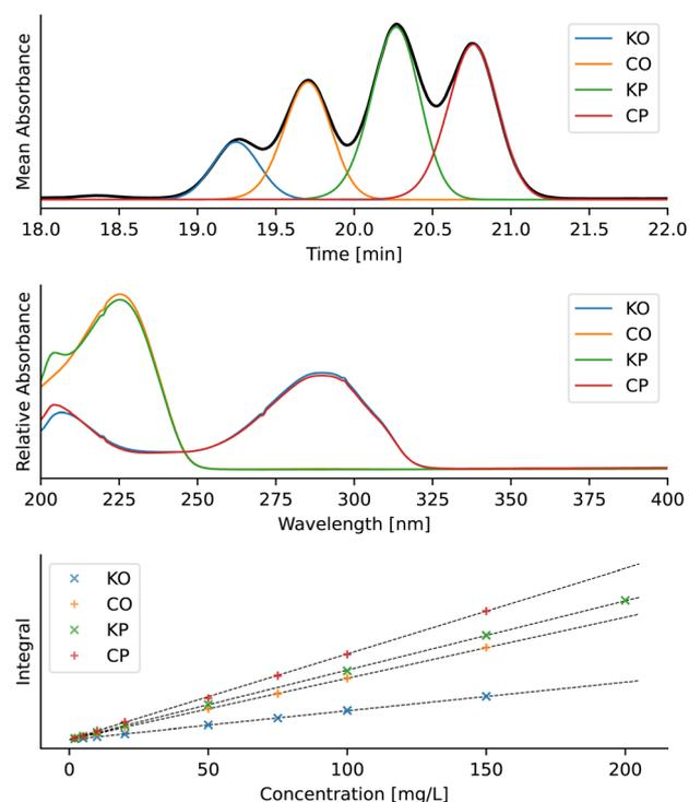
**Fig. 14** Deconvolution results of diterpene esters. From top: example of the deconvoluted chromatogram, recovered absorption spectra of individual diterpene esters, and linear calibration curves. The data in the figure are from calibration sample 16,<sup>37</sup> the baseline was corrected using FlatFit and the peaks were deconvoluted using the BEMG model. Chromatograms were analysed in the 18–22 minute interval over the entire provided UV-vis spectrum (200–400 nm).
