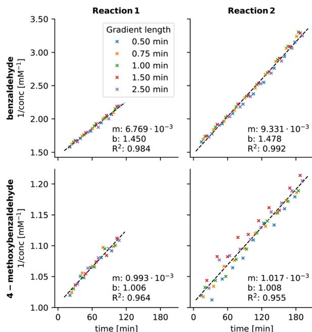
**Fig. 12** Pseudo-second order kinetic plots of **3a** and **3b** derived from competition experiments in the Knoevenagel condensation recorded with five different gradient length runs and analyzed with the new MOCCA version. Reaction 1 contains **3a** and **3b** and Reaction 2 contains **3a**, **3b** and **3c**. The data are fitted with straight line  $y = mx + b$ .
