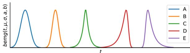
Fig. 3 Examples of possible peak shapes using the BEMG model, including different widths, symmetric distortion, fronting, and tailing. (A)  $\sigma = 0.3$ ,  $a = 100$ ,  $b = 100$ , (B)  $\sigma = 0.2$ ,  $a = 100$ ,  $b = 100$ , (C)  $\sigma = 0.05$ ,  $a = 5$ ,  $b = 5$ , (D)  $\sigma = 0.1$ ,  $a = 3$ ,  $b = 100$ , and (E)  $\sigma = 0.1$ ,  $a = 100$ ,  $b = 3$ . All peaks are normalized to have equal height.
