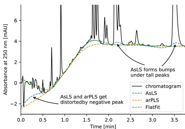
**Fig. 1** Comparison of baseline estimation using AsLS, arPLS and FlatFit algorithms on a representative chromatogram of a reaction mixture measured at 250 nm without blank subtraction. Typically, the baseline would be first corrected by subtracting a blank chromatogram and only then refined using a baseline estimation algorithm. The blank was not subtracted in this case to highlight the differences between the different algorithms.
