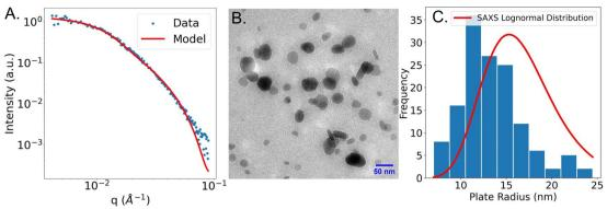
Fig. 5 This figure shows the data from the randomly chosen sample that was fit using a plate model. (A) The SAXS curve and the plate model that was used to fit the data. (B) An electron microscopy image from the set of images that were taken of the sample. (C) A histogram of the plate radii from all the images that were taken. The lognormal distribution with the plate radius and polydispersity obtained from SAXS is plotted in red.
