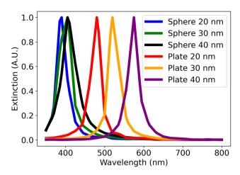
**Fig. 1** The simulated spectra of spheres and plates using nano-DDSCAT. The legend refers to the diameter of simulated the plates and spheres. All simulated plates have a thickness of 7 nm.
