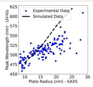
Fig. 8 The comparison between the plate radius determined by the peak wavelength position from UV-vis spectroscopy and the radius determined by SAXS. The data from the simulated plates are also plotted assuming that the radius determined from SAXS is the "true" radius.
