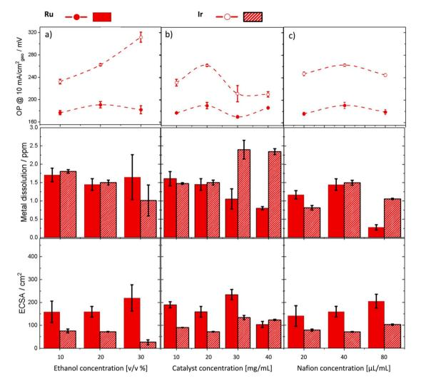
Fig. 5 Impact of varying ink formulation parameters on OER performance for Ru and Ir metals. A set of experiments showing the effect of varying (a) ethanol concentration, (b) catalyst concentration (mass loading), and (c) Nafion concentration on the overpotential (OP), metal dissolution, and ECSA of Ru and Ir. Solid circles and bars are used for Ru, and empty circles and hatched bars are used for Ir. Each experiment was repeated three times
