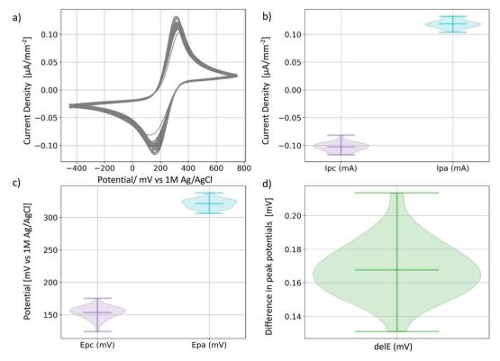
Fig. 3 Reproducibility of electrochemical testing in reactor cells. (a) 30 cyclic voltammetry tests on potassium ferricyanide  $[K_3Fe(CN)_6]$ . (b) Anodic and cathodic current density peak values,  $I_{pa}$  and  $I_{pc}$ , respectively. (c) Anodic and cathodic potential peak potential values,  $E_{pa}$  and  $E_{pc}$ , respectively. (d) Difference in potential between cathode and anode peaks.
