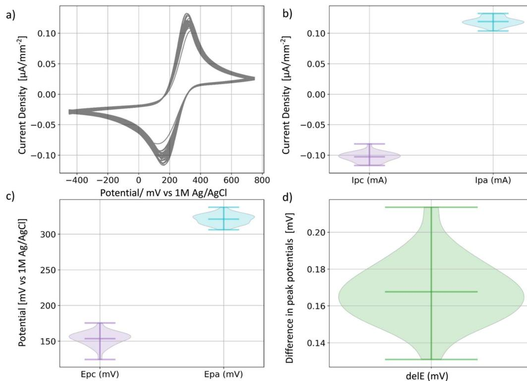
Fig. 3 Reproducibility of electrochemical testing in reactor cells. (a) 30 cyclic voltammetry tests on potassium ferricyanide [ $\text{K}_3\text{Fe}(\text{CN})_6$ ]. (b) Anodic and cathodic current density peak values,  $I_{pa}$  and  $I_{pc}$ , respectively. (c) Anodic and cathodic potential peak potential values,  $E_{pa}$  and  $E_{pc}$ , respectively. (d) Difference in potential between cathode and anode peaks.
