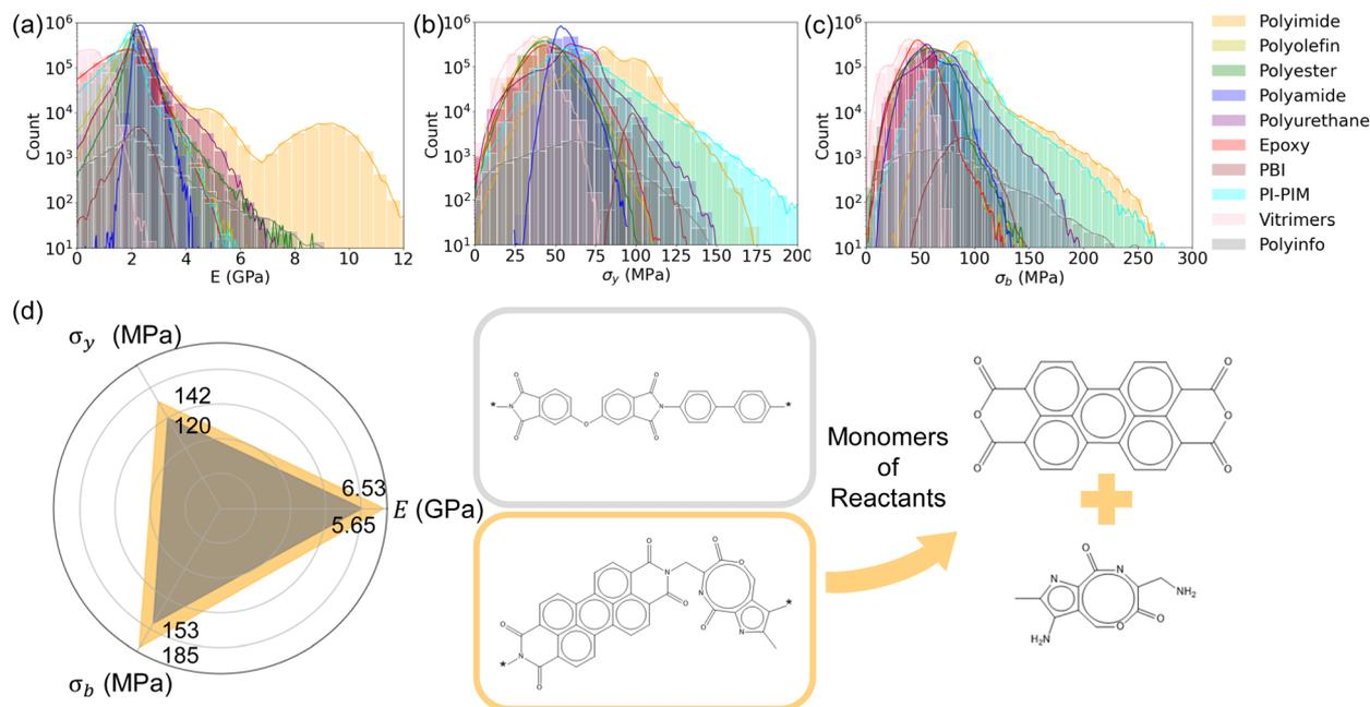
Fig. 6 Distributions of (a)  $E$ , (b)  $\sigma_y$ , and (c)  $\sigma_b$  prediction results of real polymers from the PolyInfo dataset and each kind of generated hypothetical polymer. (d) The real polymer with the highest predicted  $E$ ,  $\sigma_y$ , and  $\sigma_b$  values in the PolyInfo dataset, and a hypothetical polyimide with predicted  $E$ ,  $\sigma_y$ , and  $\sigma_b$  values exceeding this performance, along with the small molecule compounds used for its synthesis.
