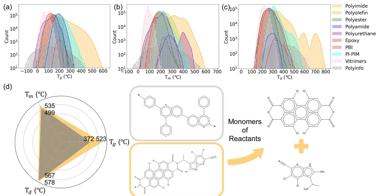
Fig. 5 Distributions of (a)  $T_g$ , (b)  $T_m$ , and (c)  $T_d$  prediction results of real polymers from the PolyInfo dataset and each kind of hypothetical polymer. (d) The real polymer with the highest predicted  $T_g$ ,  $T_m$ , and  $T_d$  values in the PolyInfo dataset, and a hypothetical polyimide with predicted  $T_g$ ,  $T_m$ , and  $T_d$  values exceeding this performance, along with the small molecule compounds used for its synthesis.
