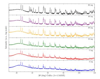
Fig. 6 XRD patterns from the different quantities of the TiO<sub>2</sub> samples (3 mg, 5 mg, 10 mg, 20 mg, 40 mg, and 80 mg) prepared by the robotic arm. The patterns are displayed on a logarithmic intensity scale.
