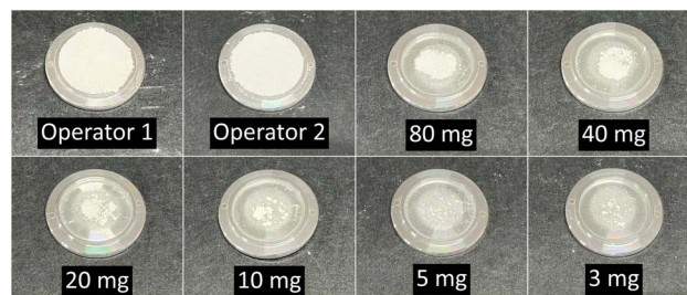
Fig. 4 Photographs of the TiO 2 samples prepared by manual operation and the robotic arm in different quantities.
