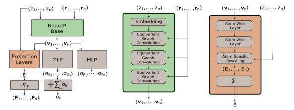
Fig. 2 The computational graph of the stochastic model for predicting the means  $\hat{E}$ ,  $\hat{F}_i$  and standard deviations  $\sigma_{E}$ ,  $\sigma_{E}$ , of the potential energy Eand atomic forces  $F_i$  from the atomic numbers  $z_i$  and coordinates  $r_i$ . The computational graph for the calculation of the means coincides with the original NegulP model, while the MLPs are modifications for modeling probabilistically.
