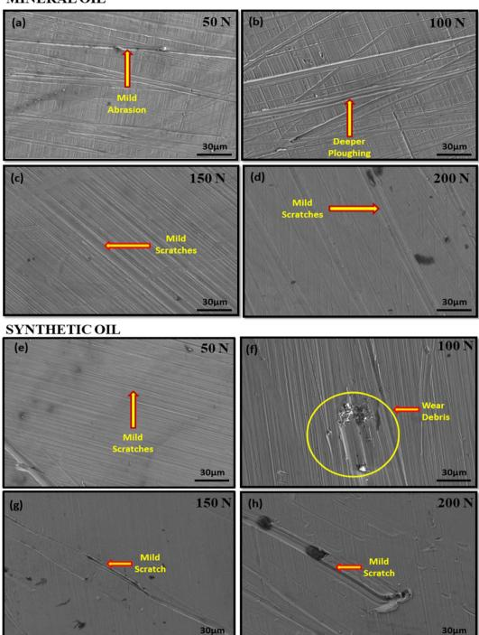
Fig. 7 Worn surface morphologies of HEA samples at (50-200 N) using mineral oil (a-d) and synthetic oil (e-h).
