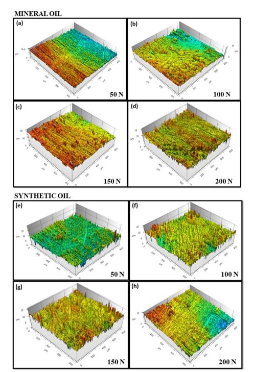
Fig. 10 3D surface roughness maps of HEA samples at 50-200 N using mineral oil (a-d) and synthetic oil (e-h).
