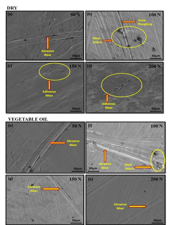
Fig. 6 Worn surface morphologies of HEA samples at (50-200 N) for dry state (a-d) and vegetable oil (e-h)
