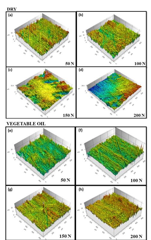
3D surface roughness maps of HEA samples at (50–100 N) for dry state (a–d) and vegetable oil (e–h).
