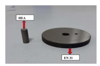
Fig. 1 Test samples used in experiments.
