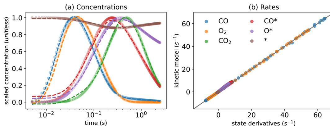
Fig. 2 KINN optimization of single-pulse CO oxidation under minimization of cost function  $J$  in eqn (4) for (a) concentrations, where circles represent target values and dashed lines represent predicted values, and (b) a parity plot of rates extracted from the KINN model and predicted from the kinetic model.
