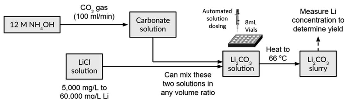
Fig. 2 Block flow diagram of the high-throughput experimentation workflow and softening process for converting  $\text{LiCl}$  to  $\text{Li}_2\text{CO}_3$  using  $\text{CO}_2(\text{g})$  and aqueous ammonium hydroxide ( $\text{NH}_4\text{OH}$ ).
