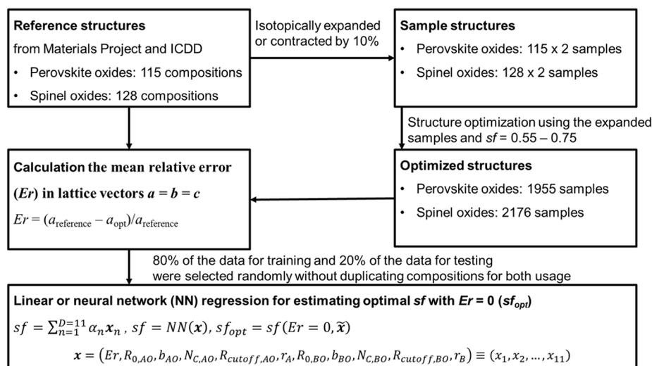
Fig. 2 The procedure of optimizing the screening factor.
