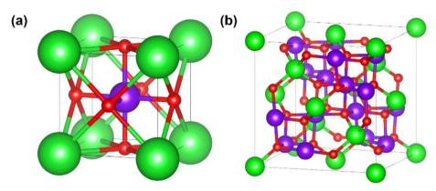
Fig. 1 Crystal structures of (a) perovskite (A – green, B – violet, O – red), (b) spinel (A – green, B – violet, O – red) oxides.
