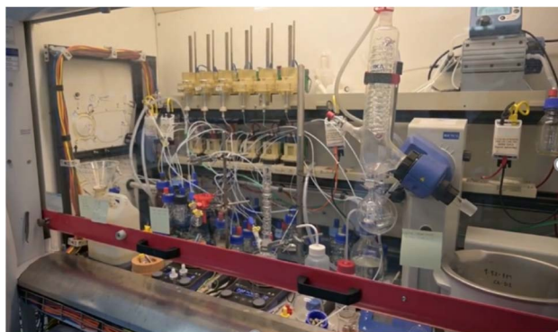
Fig. 8 A so-called Chemputer, designed by the Cronin lab. 133
