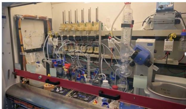
Fig. 8 A so-called Chemputer, designed by the Cronin lab.<sup>133</sup>
