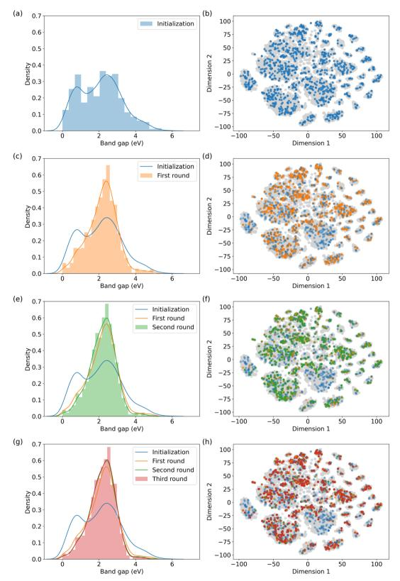
Fig. 4 MOF recommendations in QMOF database based on the specified band gap range. (a), (c), (e), and (g) depict the normalized distribution of band gaps of the selected MOFs in each round; and (b), (d), (f), and (h) show their positions in the chemical space, respectively. The distributions of the recommendation rounds show a peak in the specified band gap range, indicating the success of the model recommendation in locating MOFs similar to those of the candidates from the previous round.
