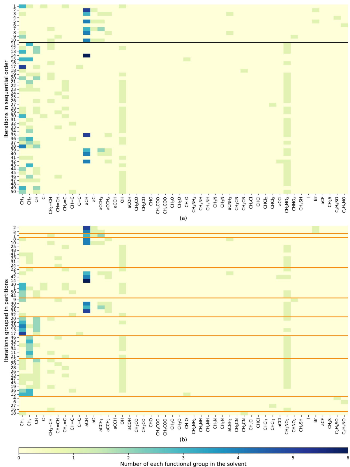
Fig. 14 Solvents identified by PWAS in 50 iterations, whose structures are depicted in functional group representations. (a) In sequential iteration order, with a black line separating the initial and active-learning samples; (b) grouped in partitions, with orange lines representing the boundary of the partitions (in total 10 partitions).
