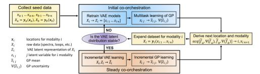
Fig. 1 Working schematics of multimodal co-orchestration.
