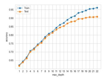
Fig. 4 Accuracy vs. max\_depth for the five-feature random forest classifier for Dataset 4, which indicates the onset of overfitting. Note how the divergence between training and testing accuracy is slower for a reduced number of features in comparison to when all features are included as in ESI, Fig. 4.
