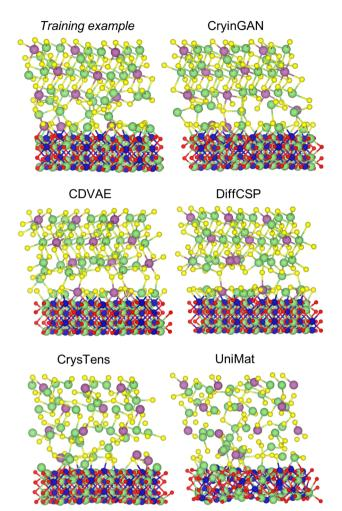
Fig. 2 Example disordered LSC-LCO interface structures generated by the generative models. The structures shown are as-generated by the models (i.e., no post-processing or relaxation). An example structure from the training dataset is also included for reference.
