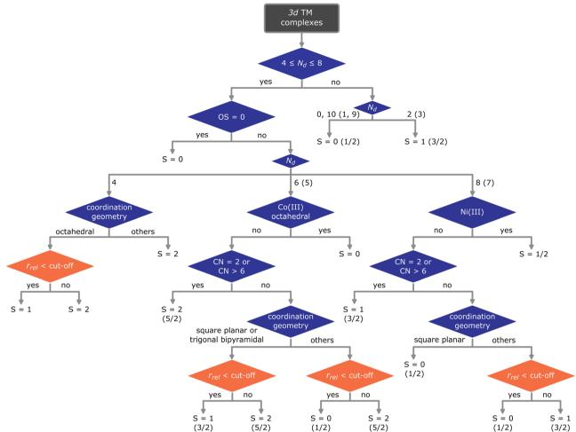
Fig. 4 Ground state spin assignment of first row TM complexes based on empirical rules.  $N_d$ : the number of d electrons, with odd numbers of d electrons shown in parentheses, OS: metal oxidation state, CN: coordination number, r<sub>rel</sub>: relative metal radius, cut-off: predefined cut-off value used to distinguish the lowest spin state. Decision nodes in orange use cut-off values that are specific for a given metal and coordination geometry (see Table S10 in the ESI†).
