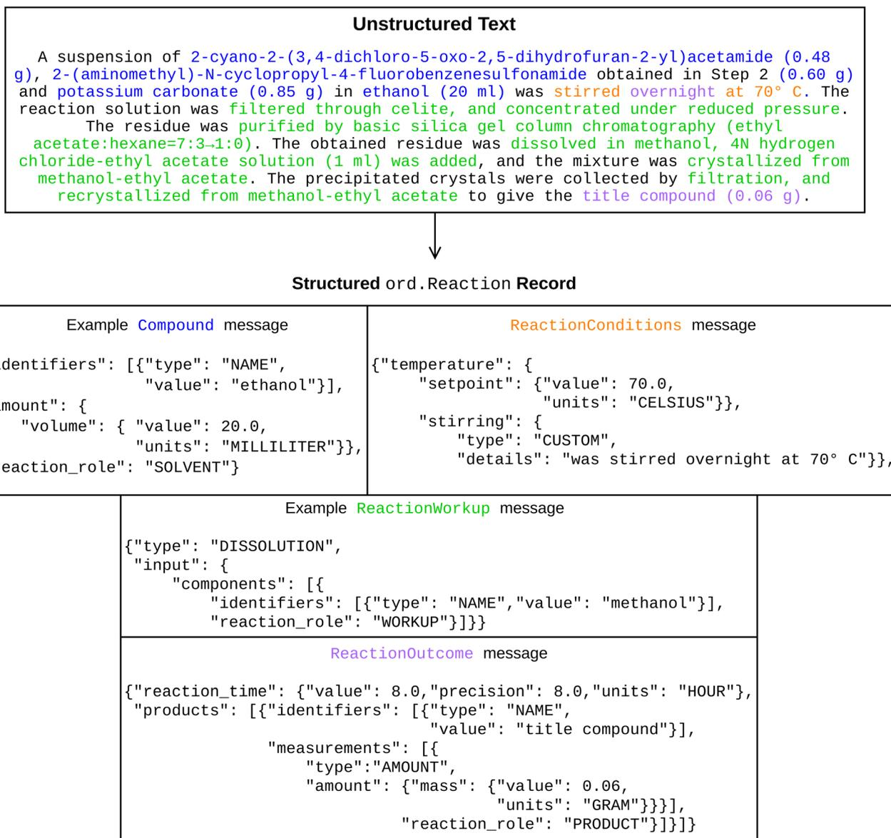
Fig. 2 (Top) The original text description of a reaction procedure and (bottom) example messages within the structured ORD reaction record.<sup>43</sup>
