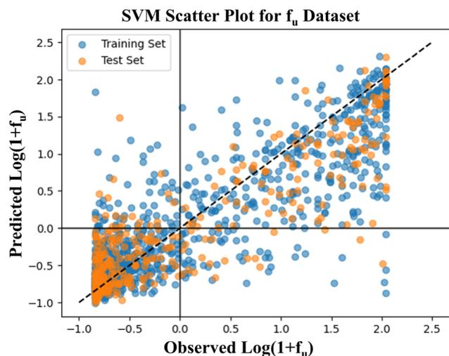
Fig. 2 Observed vs. predicted  $\log(1 + f_u)$  scatter plot for the SVM model.
