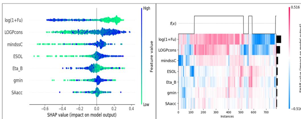
Fig. 9 SHAP plots for the SVM model (for modeling  $Cl_{int}$  by taking  $f_u$  as a descriptor).
