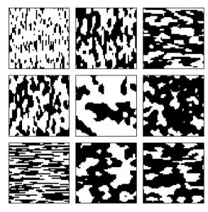
Fig. 5 Example microstructures generated for the 2D elastic property active learning workflow. Each microstructure is of size  $51 \times 51$  pixels. In this work, lamellar-like microstructures are aligned in either vertical or horizontal directions.
