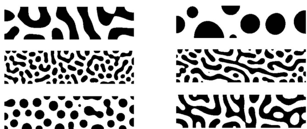
Fig. 4 Example microstructures generated for the OPV active learning workflow. Each microstructure is of size 401 \times 101 pixels.
