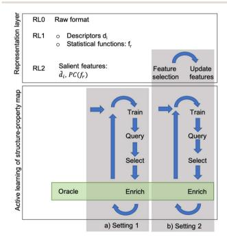
Fig. 1 Workflow: given the dataset of L microstructures and two representations (vector of descriptors and two-point correlations), find the salient features of the target properties and the associated SP relationship using active learning.
