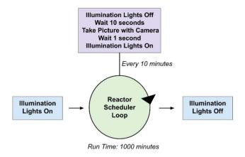
Fig. 5 Block diagram detailing the flow of commands for the  $\rm H_2$  evolution photoreactor code.
