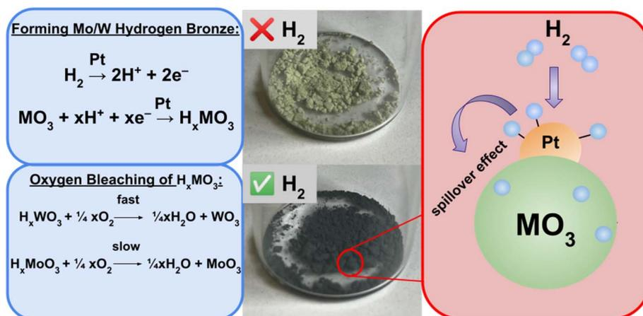
Fig. 2 Platinum catalyzed reduction of a metal oxide (M = tungsten or molybdenum) to form deep blue colored tungsten/molybdenum bronze (H<sub>x</sub>MO<sub>3</sub>) and its much slower reverse reaction (left). Images of the hydrogen sensing material in the presence and absence of H<sub>2</sub> (middle). Depiction of the dissociation of H<sub>2</sub> on the surface of the platinum catalyst and subsequent spillover of hydrogen atoms into the metal oxide lattice (right).
