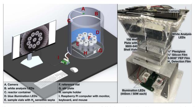
Fig. 4 Visual rendering of H<sub>2</sub> evolution photoreactor and its labeled parts (left). A picture of the wiring of the reactor set up can be found in the ESI (Fig. S1†). Labeled image of a multiwell plate hydrogen evolution photoreactor (right). Design files for this setup can be found in a previous publication.31
