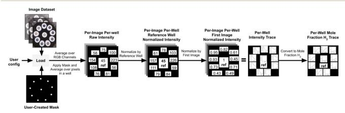
Fig. 6 Block diagram detailing the flow of commands for the H<sub>2</sub> evolution photoreactor code.
