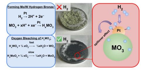
Fig. 2 Platinum catalyzed reduction of a metal oxide (M = tungsten or molybdenum) to form deep blue colored tungsten/molybdenum bronze (H<sub>x</sub>MO<sub>3</sub>) and its much slower reverse reaction (left). Images of the hydrogen sensing material in the presence and absence of H<sub>2</sub> (middle). Depiction of the dissociation of H<sub>2</sub> on the surface of the platinum catalyst and subsequent spillover of hydrogen atoms into the metal oxide lattice (right).
