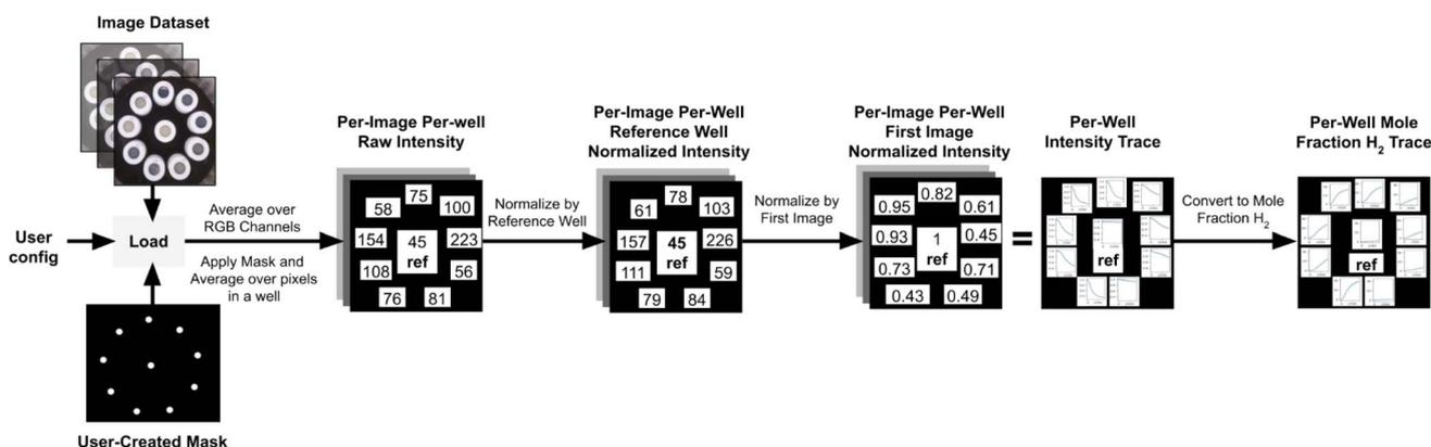
Fig. 6 Block diagram detailing the flow of commands for the H<sub>2</sub> evolution photoreactor code.
