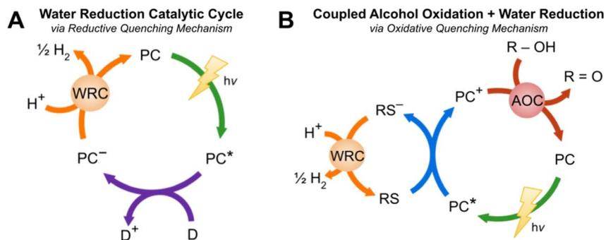
Fig. 1 (A) Light-driven water reduction catalytic cycle<sup>14</sup> for the photogeneration of H<sub>2</sub> proceeding via a reductive quenching mechanism composed of a PC, D, and WRC. (B). Photo-driven coupled alcohol oxidation and water reduction catalytic cycle<sup>14</sup> via an oxidative quenching mechanism containing a PC, RS, WRC, AOC, and R-OH.
