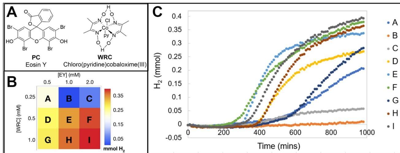
Fig. 10 (A) Structures of the PC and WRC used in experiment 1. (B) Array plot of the maximum H<sub>2</sub> evolved and reaction conditions for all samples in experiment 1. (C) H<sub>2</sub> evolution traces for experiment 1.
