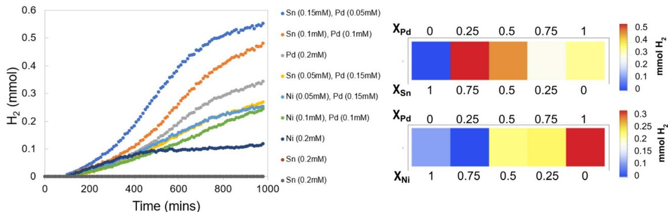
Fig. 12 H<sub>2</sub> evolution traces for experiment 3 (left), and array plots of overall H<sub>2</sub> evolution at different metal incorporations (right).
