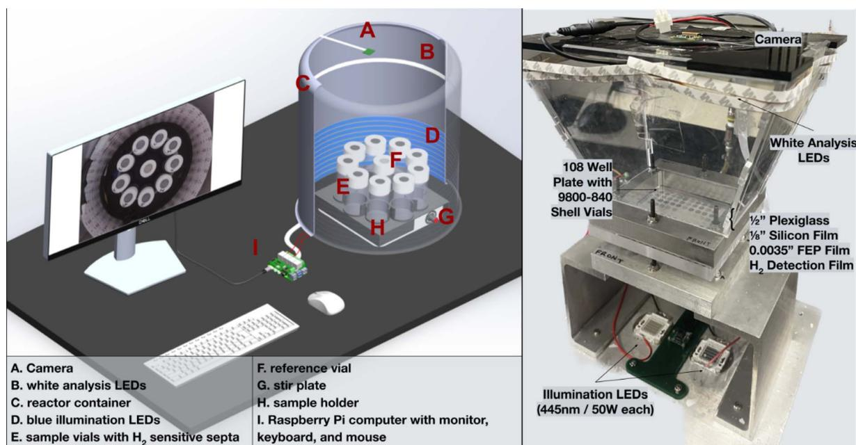
Fig. 4 Visual rendering of H<sub>2</sub> evolution photoreactor and its labeled parts (left). A picture of the wiring of the reactor set up can be found in the ESI (Fig. S1†). Labeled image of a multiwell plate hydrogen evolution photoreactor (right). Design files for this setup can be found in a previous publication.<sup>31</sup>
