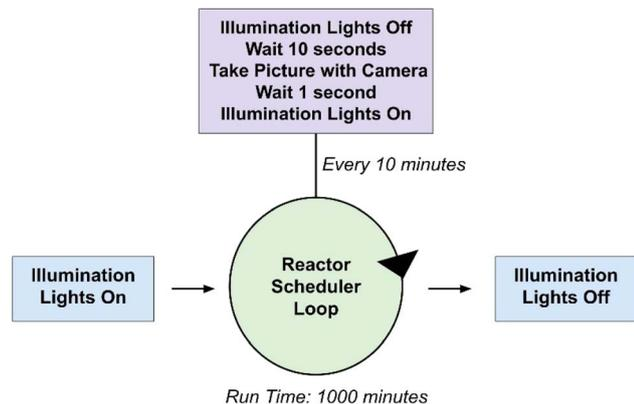
Fig. 5 Block diagram detailing the flow of commands for the H<sub>2</sub> evolution photoreactor code.
