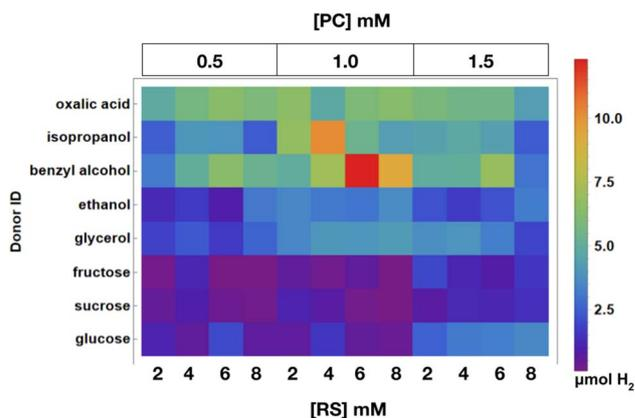
Fig. 13 Array plot displaying the total H<sub>2</sub> evolved for eight different donor species at three different photocatalyst concentrations and four different RS concentrations. Substrates that are easier to oxidize exhibit a quicker onset of hydrogen production and generally produce higher yields of photogenerated H<sub>2</sub>.
