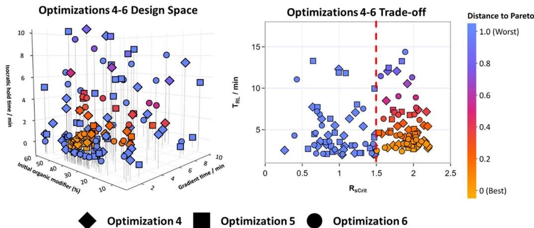
Fig. 5 The design spaces for optimizations 4–6 and the trade-off between  $R_{sCrit}$  and  $t_{RL}$  where  $N = 7$ . The color scale represents the distance to Pareto front when  $R_{sCrit} \geq 1.5$ , represented by points to the right-hand side of the dotted line in the trade-off plot.
