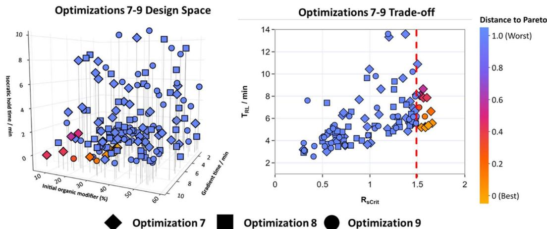
Fig. 6 The design spaces for optimizations 7–9 and the trade-off between  $R_{s,Crit}$  and  $t_{RL}$  where  $N = 11$ . The color scale represents the distance to Pareto front when  $R_{s,Crit} \geq 1.5$ , represented by points to the right-hand side of the dotted line in the trade-off plot.
