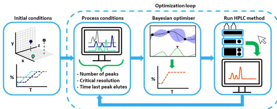
Fig. 1 A schematic of the closed loop HPLC method optimization system.
