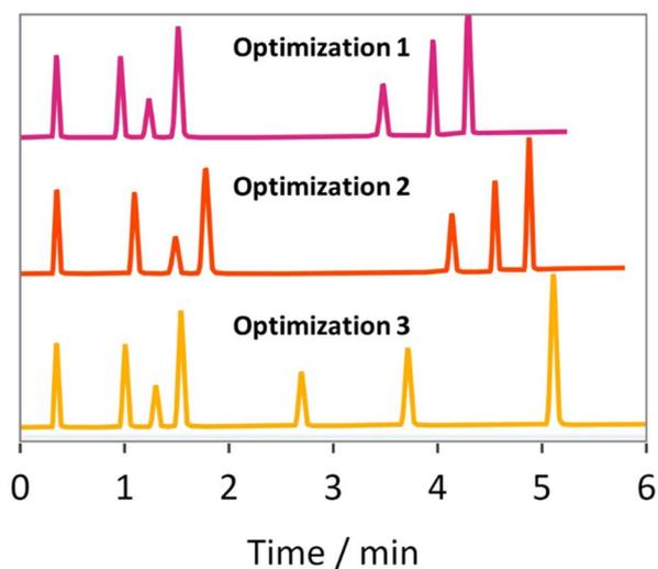
Fig. 3 The first chromatograms from optimizations 1 (top), 2 (middle) and 3 (bottom) that satisfied the design space criteria ( $N = 7$ ,  $R_{sCrit} \geq 2$  and  $t_{RL} \leq 6$  minutes), representing experiments 12, 19 and 9 respectively.
