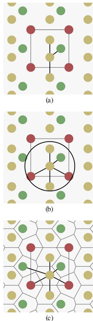
Fig. 1 Edge selection for a single atom in a crystal structure. Red atoms mark the cubic unit cell. Depicted edge selection methods are  $k$ -nearest neighbors ( $k$ NN) in (a), cut-off radius in (b) and Voronoi diagram in (c).
