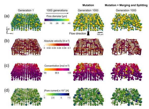
Fig. 3 The geometrical evolution of cubic networks with only a mutation operator, and a combination of a mutation and a merging and splitting operator. The networks of the first and final (1000th) generations are shown, displaying the: (a) pore diameter evolution, (b) the throat absolute velocity, (c) the reactant pore concentration, and (d) the absolute pore current. With the flow in the *y*-direction and the thickness in the *z*-direction with the membrane facing to the top.
