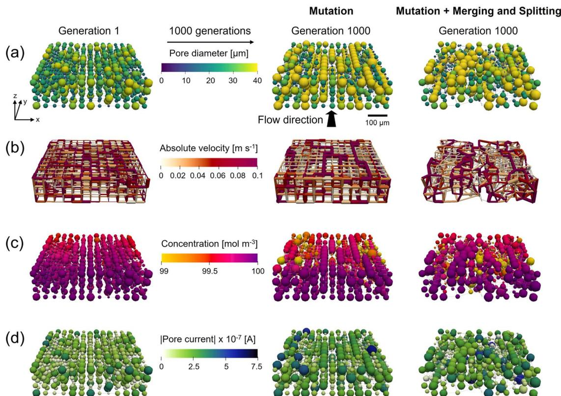
**Fig. 3** The geometrical evolution of cubic networks with only a mutation operator, and a combination of a mutation and a merging and splitting operator. The networks of the first and final (1000th) generations are shown, displaying the: (a) pore diameter evolution, (b) the throat absolute velocity, (c) the reactant pore concentration, and (d) the absolute pore current. With the flow in the  $y$ -direction and the thickness in the  $z$ -direction with the membrane facing to the top.
