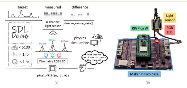
Fig. 5 The CLSLab:Light demo. (a) A summary schematic of CLSLab:Light. (b) An annotated image of the CLSLab:Light. (c) Was adapted with permission from ref. 65. Copyright Elsevier 2022.
