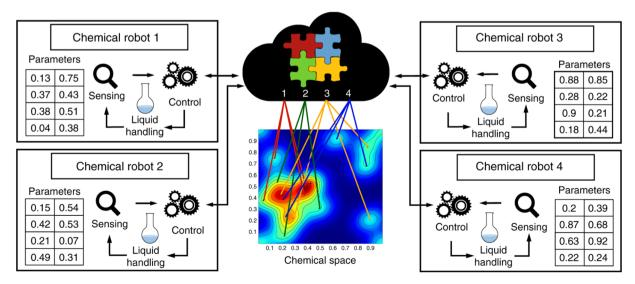
Fig. 12 Illustration of a network of parallel chemical synthesis robots working towards a common optimization goal.<sup>75</sup> Reproduced from ref. 73 with permission under the Creative Commons Attribution license (CC-BY). Copyright © 2018, Caramelli et al.
