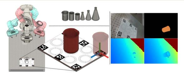
Fig. 11 April Tags, a type of fiducial marker, are affixed to a base plate to allow for accurate detection of its position and orientation (six degrees of freedom) relative to the camera. Reproduced from ref. 122 with permission from H. Xu, Y. R. Wang, S. Eppel, A. Aspuru-Guzik, F. Shkurti and A. Garg, arXiv, 2021, https://doi.org/10.48550/arXiv.2110.00087.
