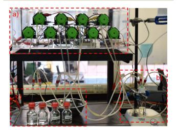
Fig. 2 MIK-I, a low-cost automated synthesis workflow platform. (a) Peristaltic pumps controlled by a Raspberry Pi, (b) synthesis reactor, (c) reagent bottles.<sup>72</sup>
