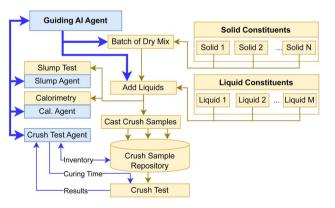
Fig. 2 A representative schematic showing the connection between different stages of the physical platform and the ML with three representative measurement modalities. Blue lines represent data flow brown lines represent physical material flow. The blue agents are responsible for measurement control, sample tracking, and data analysis.
