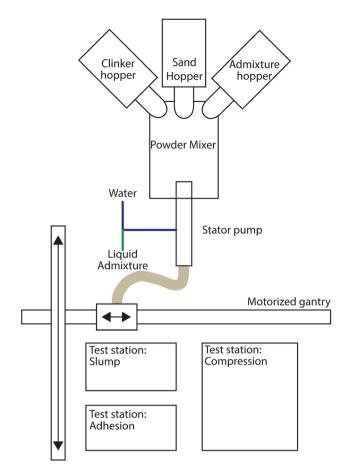
Fig. 1 Cartoon schematic showing the layout, viewed from above, of the described automated synthesis and characterization platform. System complexity can be scaled up or down depending on the scope of the research
