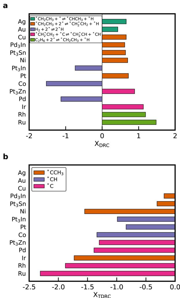
Fig. 6 (a) Elementary reaction with the highest degree of rate control  $X_{DRC}$  and (b) adsorbate with the highest thermodynamic degree of rate control  $X_{TDRC}$  for each metal. Metals are sorted according to the carbon binding energy going from weakest (Ag) to strongest (Ru). There is no species with a significant TDRC for Ag, Au, Cu, because the surface is vacant under the operating conditions.
